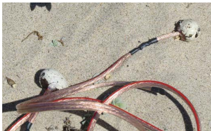
Figure 14: Two electrified eggs each connected to the network of speaker wires connecting all the electrified eggs to each other and the shocking unit. The connection of the electrified eggs to the network of speaker wires was soldered and covered with a heat shrink tube.
