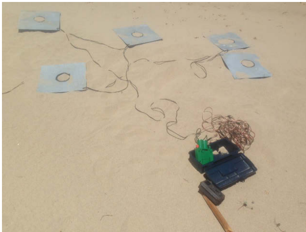
Figure 17: Steel plates and shocking unit with attached wires, laid on top of the sand prior to burying the items underneath the sand. The game camera fixed on the wooden stake laid on the sand prior to deployment.
